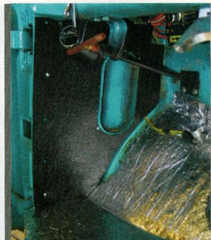
Kick panels attach with interior-style finish screws provided in the kit, as shown. These panels can be upholstered or left as is, depending on how you plan on finishing your interior.
